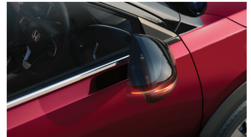
Auto-Fold Door Mirrors with LED Turn Signal
